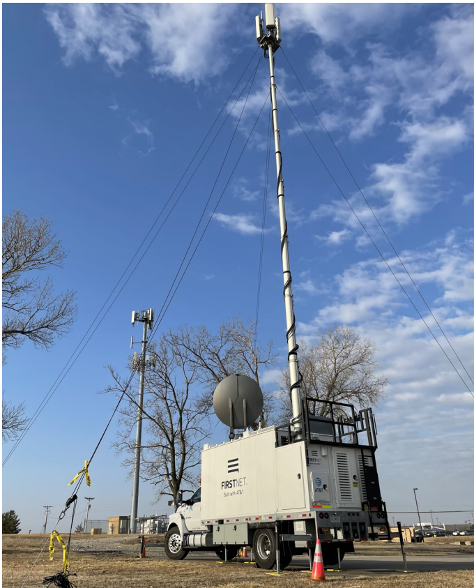
Sat-Colt (Satellite Cell on Light Truck) deployed for a local tower outage. Moline, IL 2022.
